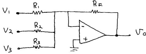
$$\frac{V_o}{R_F} + \frac{V_1}{R_1} + \frac{V_2}{R_2} + \frac{V_3}{R_3} = 0$$
