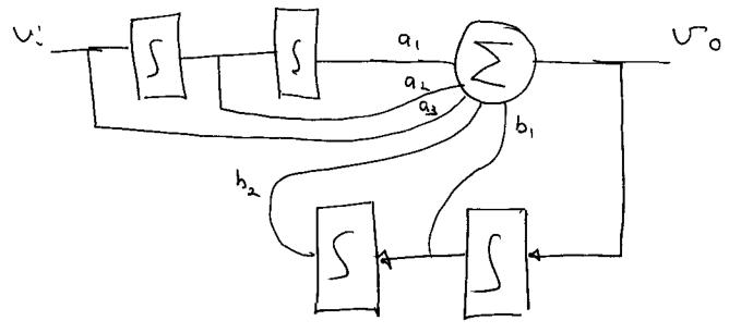
$$V_0 = \frac{a_1 V_1}{5} + \frac{a_2 V_1}{5^2} + \frac{a_3 V_1}{5} + \frac{b_1 V_0}{5} + \frac{b_2 V_0}{5^2}$$
